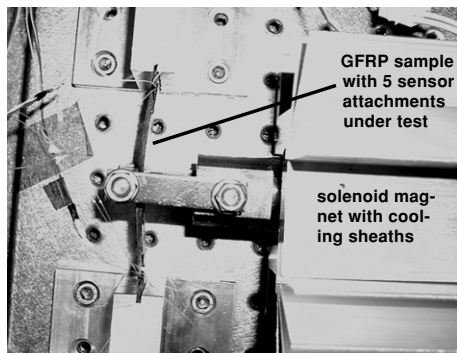
Figure 5. Photograph of the test set for application of periodic strain loads. Maximum strain cycle rate: 50 \text{ s}^{-1} . Maximum strain amplitude: 2000 \mu\epsilon .
