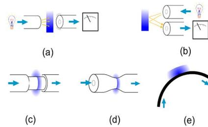
Fig. 14. Generic configurations of optical fiber sensors for chemical sensing in structural health monitoring: extrinsic transmissive (a) and reflective (b), with a stripped cladding (c), a taper (d), or with a curvature in the fiber (e).
