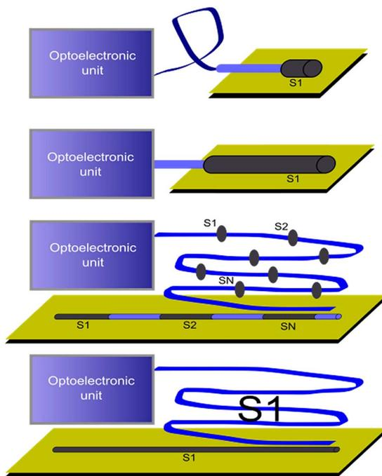
Fig. 5. Optical fiber sensor types according to the spatial distribution of the measurands: (a) point; (b) integrated; (c) distributed; (d) quasi-distributed.
