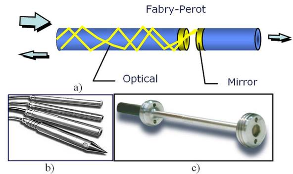
Fig. 12. Schematic illustration of an EFPI transducer used for both chemical and physical point transducers (a). Commercial transducer for pressure (b) and strain (c). Courtesy of Roctest.
