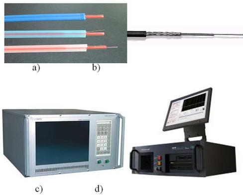
Fig. 11. Two commercial transducers (aforementioned) and two optoelectronic units (in the following). Fiber transducers for both temperature and strain (a), for temperature (b). DiTest Brillouin (c) and Raman (d) scattering interrogation units. Courtesy of Smartech, Omnisens and Sensornet.
