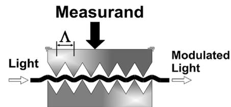
Fig. 13. Point transducer based on periodic microbends.
