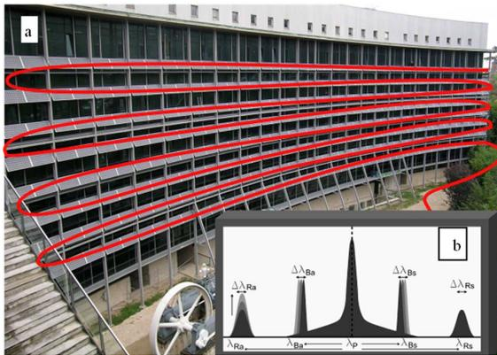
Fig. 9. Distributed temperature fiber Sensor illustrated on the front wall of the Ind. and Telecommunications School at the University of Cantabria, UC. (a) Distributed transducer (red color). (b) Optoelectronic Unit, OU. Courtesy of the Photonic Engineering Group of UC.
