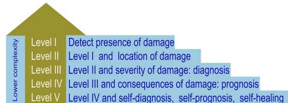
Fig. 2. Staircase of the SHM: levels in Health Monitoring systems. Higher the level, the higher the complexity.
