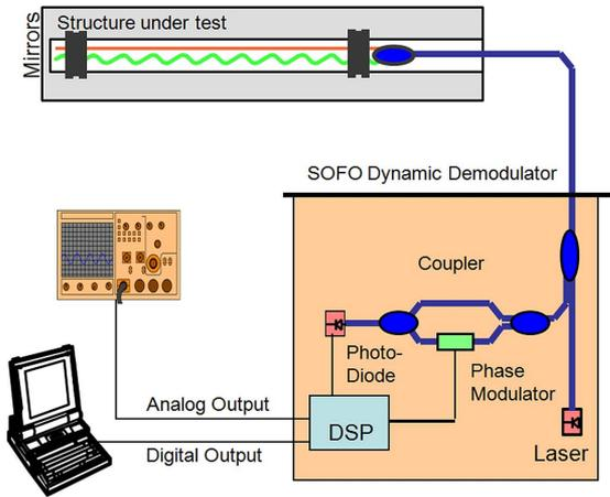
Fig. 6. Conceptual illustration of SOFO Dynamic. Courtesy of Smartec.
