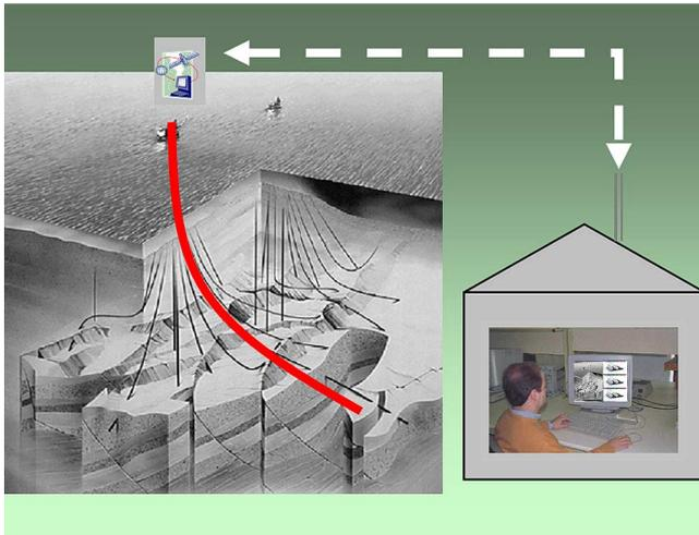
Fig. 19. *Smart well and field* concept illustration in an off-shore oil field. Measurand data are obtained in real time or in quasi-real time and it can be made available in the central monitoring office. Appropriate reactions or actuations may even be done, automatically.
