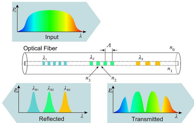
Fig. 7. Illustration of the fiber Bragg grating concept and its optical function. It should be noted that  $\lambda_{Bx} = 2n_{\text{eff}x}\Lambda_x$ .
