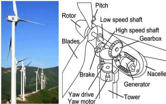
Fig. 16. Wind turbine and details of key subsystems to be monitored. Photo courtesy of COPSESA.
