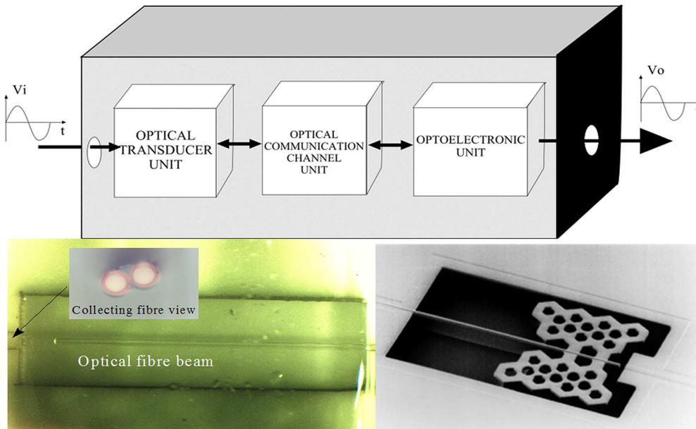
Fig. 4. Main blocks of an OFS (upper). Very low-frequency accelerometer transducers in fiber and Integrated Optic technologies developed in the framework of the European Brite Euram 7289 project (Lower). Courtesy of Photonics Engineering Group of the University of Cantabria and CEA-LETI, Grenoble, France, respectively.
