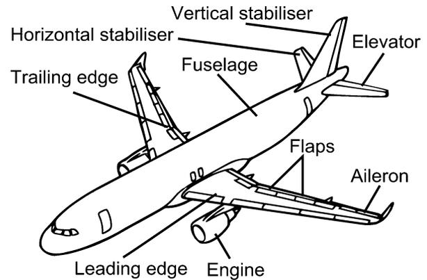
Fig. 17. Illustration of key parts of a typical aircraft to be monitored.
