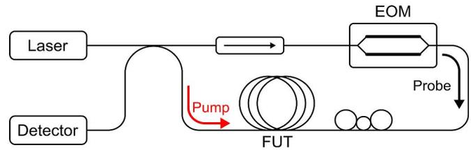
Fig. 10. Illustration of a basic setup scheme for BOTDA.
