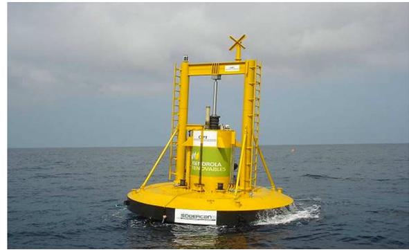
Fig. 15. Sea-wave turbine in experimental phase in Santoña Spain. Placed at 10 km from the coast, the device converts the vertical movement of the sea waves into electric energy by means of a conventional generator. Courtesy of Sodercan.
