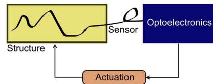
Fig. 1. Illustration of the concept of a general SHM system.
