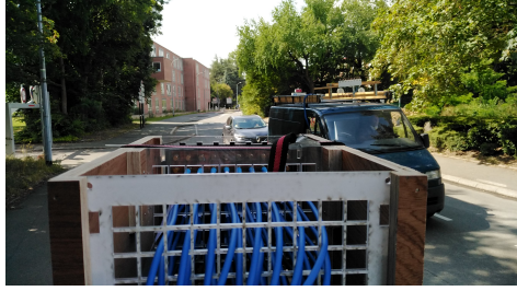
Fig. 3. Picture from the rear side of the Tx array with the van completing its drive test. The Rx antenna is one of the 8 antennas located on the van rooftop.
