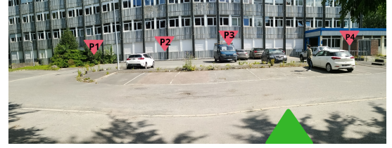
Fig. 4. Schematic top view of the 4 OLOS static measurement positions. The green triangle corresponds to the Tx position on the sidewalk behind the trees observable by their shadows on the ground.
