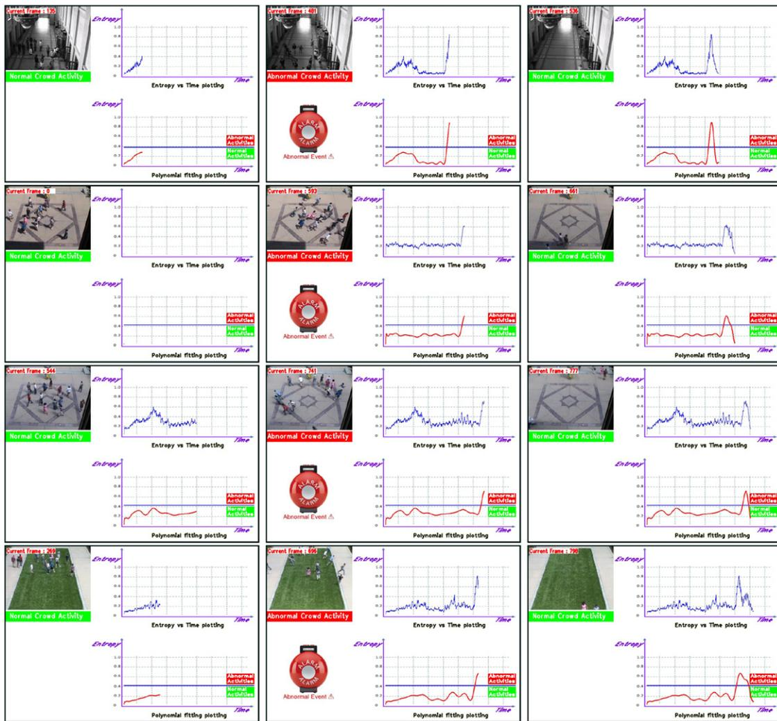
Fig. 16. Qualitative results of abnormal behaviors detection using the proposed framework for the same four sample videos as demonstrated in [19] from the UMN dataset.
