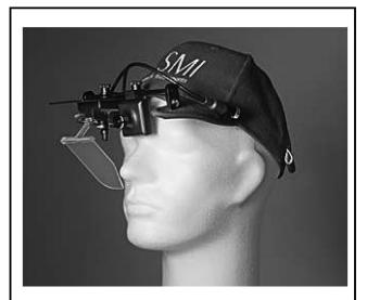
**FIGURE 2.** Picture of the head mounted eye-tracker that we used.
