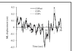
**FIGURE 3.** Time series for COPnet, COP $\nu$ , and COPc in one trial (30 s long) performed by the experimenter (units: cm) in the medialateral (ML) axis. The COPnet is the integrated displacement of the COP under both feet. The COP $\nu$ (t) is the component of the COPnet(t) that can be explained by the bodyweight mechanism. The COPc(t) is the component of the COPnet(t) that can be explained by the center of pressure location mechanism.
