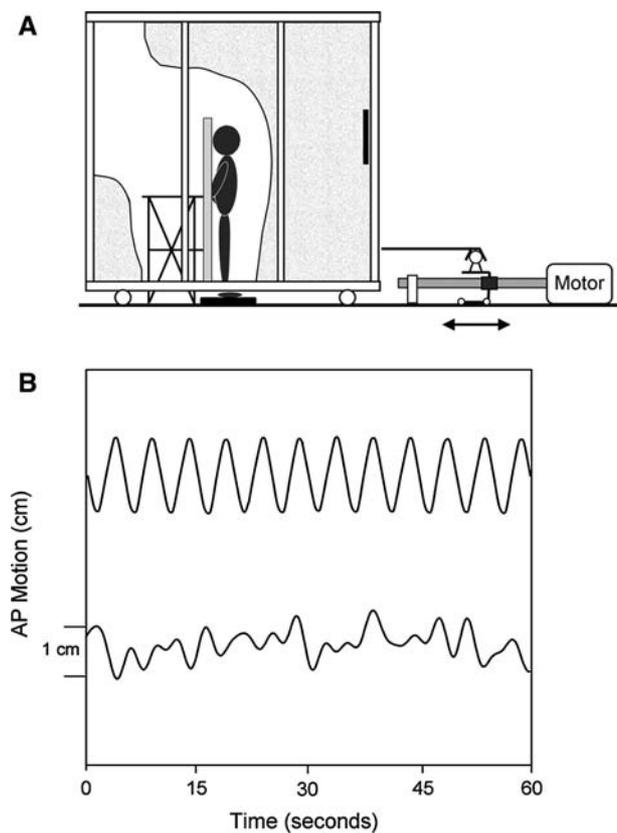
**Fig. 1** **a** The moving room and the tilt table. **b** Motion patterns of the moving room. Upper trace: Motion at 0.2 Hz with amplitude 1.5 cm and duration 60 s. Lower trace: A portion of the sum-of-sines stimulus, which continued for 600 s without repeating. The maximum amplitude of the sum-of-sines was 1.8 cm
